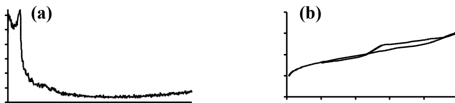
Figure SI 4. (a) X-ray diffraction pattern and (b) nitrogen sorption isotherm of MSN loaded with cytochrome c (95 mg/g).
